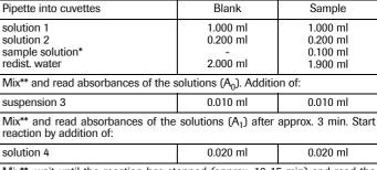
Mix\*\*, wait until the reaction has stopped (approx. 10-15 min) and read the absorbances of the solutions (A<sub>2</sub>). If the reaction has not stopped after 15 min, continue to read the absorbances
