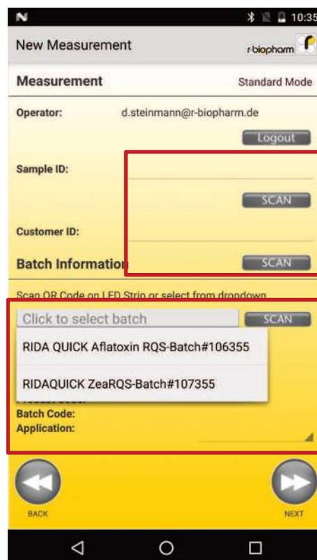
It is important to define the Sample (**Sample ID**) before performing a new measurement. It is possible to manually enter this data or to scan a barcode when available. The Customer (**Customer ID**) is optional
