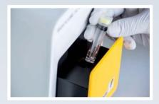
Close the tube with the cap and insert the cartridge into the instrument
