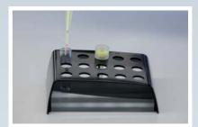
Pipette the sample into the tube
