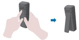
To close the stand, press the lower end of the stand to the original position.
