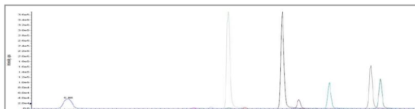
Figure 1: Example chromatogram of small animal forage spiked at EU legislative levels
