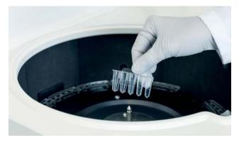
Our reagents are washed out of the cuvettes after the end of the reaction. After drying the cuvettes, they are available for further analyses (reusable cuvettes).
