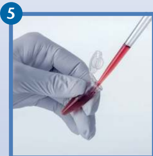
5 Remove the supernatant carefully and completely from the opposite side
