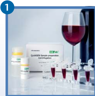
1 Add 1 mL wine into a conic (not round shaped) 1.5 mL tube
