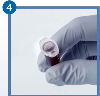
4 The non visible pellet will be at the side with the joint of the lid
