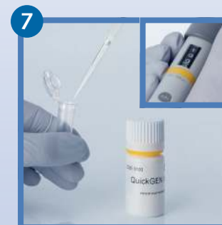
7 Add 100 µL Lysis buffer and mix/vortex: the DNA is ready to use
