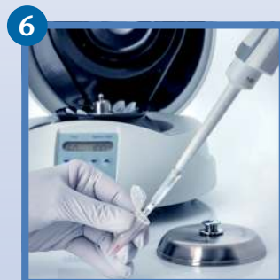
6 Start a short centrifugation spin and remove the remaining liquid completely without touching the pellet
