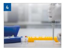
Transfer 5 µL DNA samples (controls) to 20 µL master mix
