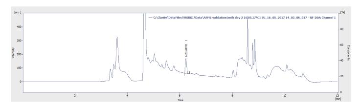
• Example HPLC Chromatogram for Powdered Milk (Spiked at 0.05 ppb)
