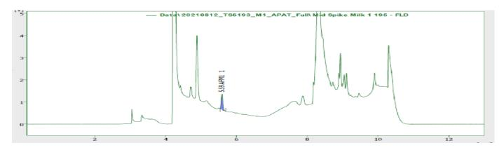
• Example HPLC Chromatogram for Milk Powder (Spiked at 0.05 ppb)
