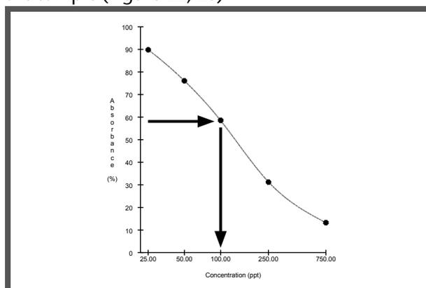
Fig. 23: A meat sample was concentrated by factor 2 during sample preparation. The result has to be multiplied with 0.5 to obtain the correct concentration: The concentration of the analyte in the sample is  $100 \text{ ng/kg} \times 0.5 = 50 \text{ ng/kg}$ .
