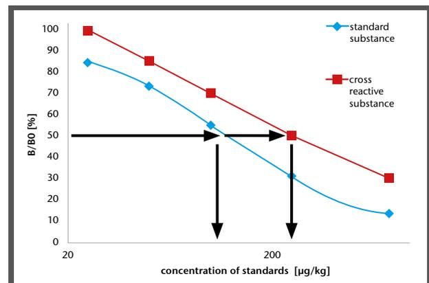
Fig. 27: The 50%-dose of the standard curve of the standard substance (blue) is more sensitive (170 µg/kg) as the 50%-dose of the standard curve of the cross reactive substance (210 µg/kg).
