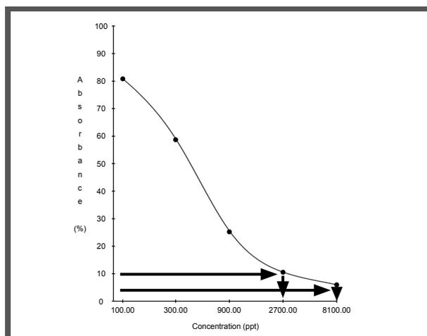
Fig. 26: In flat areas of the standard curve small differences in B/B0 produces large differences in concentration: 5 % B/B0 gives an 3 times higher results as 10 % B/B0.
