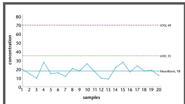
Fig. 25: 20 blank samples were analyzed. Mean of blank samples = 18 ng/kg with a standard deviation of 5,7 ng/kg
