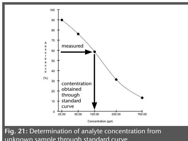
Fig. 21: Determination of analyte concentration from unknown sample through standard curve
