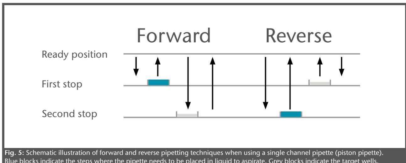
Fig. 5: Schematic illustration of forward and reverse pipetting techniques when using a single channel pipette (piston pipette). Blue blocks indicate the steps where the pipette needs to be placed in liquid to aspirate. Grey blocks indicate the target wells.
