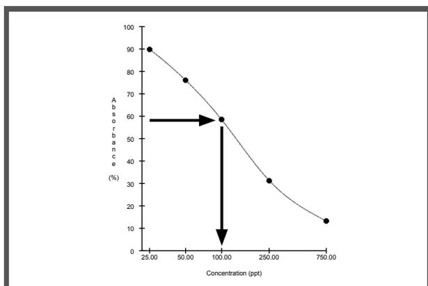
Fig. 22: A milk sample was diluted 1:4 before applying to the microtiter well. The results have to be multiplied by 4 to obtain the correct concentration: The concentration of the analyte in the sample is  $100 \text{ ng/kg} \times 4 = 400 \text{ ng/kg}$ .
