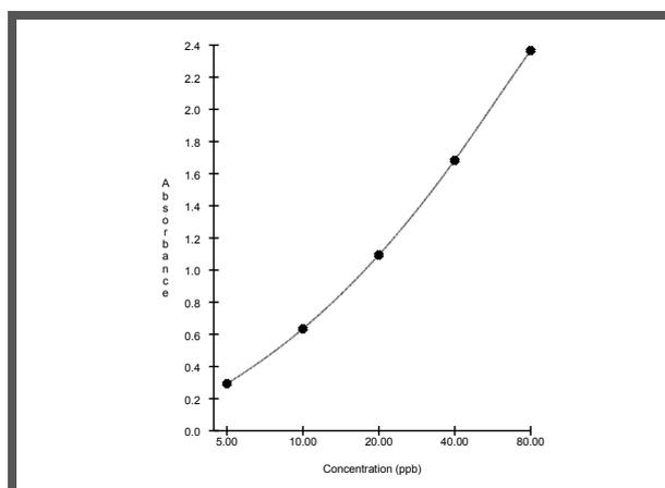
Fig. 17: Standard curve of an ELISA in sandwich format, where absorbance is plotted over concentration.
